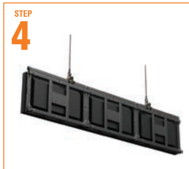
Hoist first tier above assembly area
